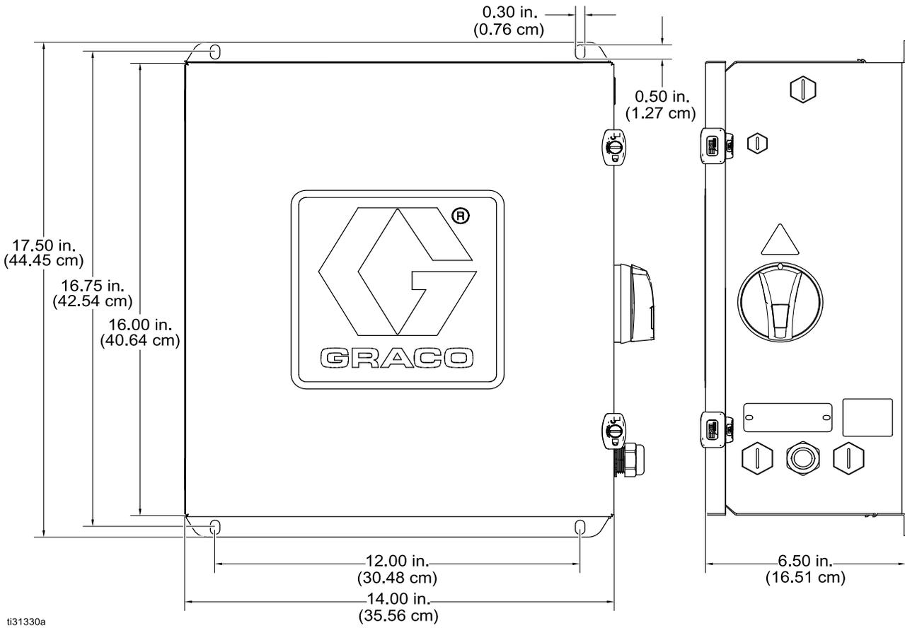
**Fig. 6 AC Control Box Dimensions and Mounting Hole Locations**
